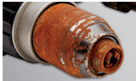
Rusted chuck – left out in the elements
