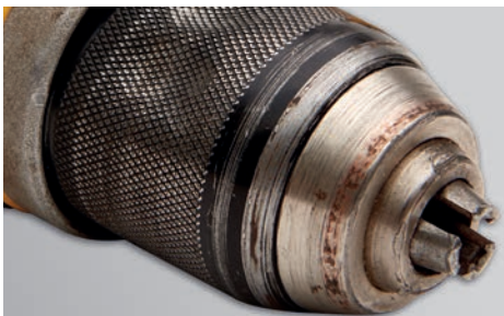
Damaged chuck – tool not taken care of
